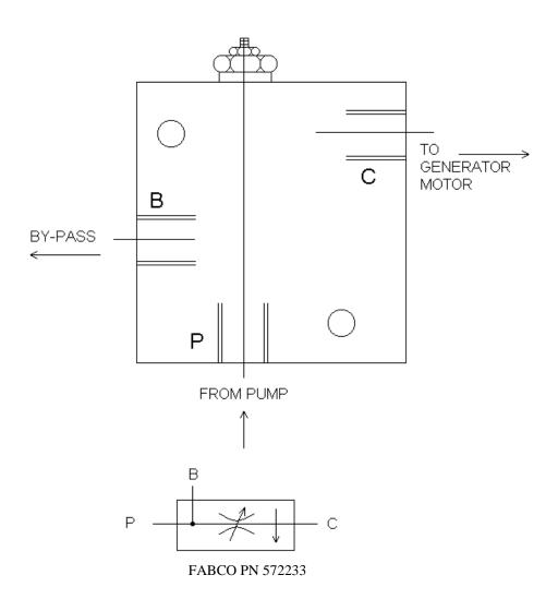
NOTE: THIS ASSEMBLY ONLY NEEDED WITH FIXED DISPLACEMENT TYPE GEAR PUMP.
